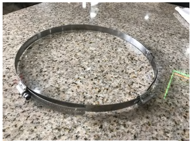
This may just look like several band clamps joined together but it's actually a very handy tool for holding drum brake shoes in place while you attach the hold-down hardware. Thanks Sal Difabio.
